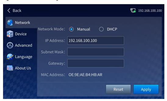
The device supports both automatic (DHCP) and manual IP configuration. When the device is connected via router or switch, DHCP is recommended. The router or switch will automatically assign IP address to the device. When the network mode is set to **Manual**, you need to set **IP Address**, **Subnet Mask** and **Gateway**.
