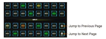
The input source page turning button supports cyclic page turning.
