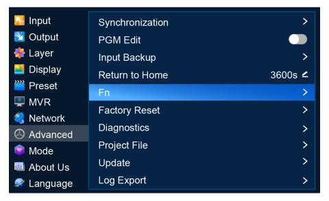
Select **Fn** to access the submenu. Select **Synchronization**, **Freeze**, **FTB**, **Test Pattern** or **Capture** to assign the selected function to the FN button.
